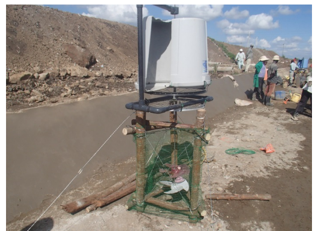
ECO-FAN at the leachate treatment pond. ECO-FAN is produced with recycled materials such as a dust bin, bicycle wheels and fans from the electric fan. Even a breeze will rotate the fans and enhance aeration of leachate to be accumulated in the pond
